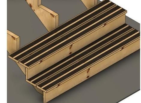
5. Then, place the top stringers on the support and slide the stairs perfectly in position.
