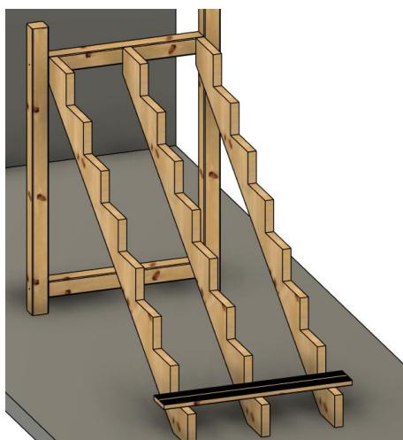
3. Screw the first plank on the first step with the RT-UT 5x60mm screws supplied with your kit. (Use 2 screws per plank and two planks per stringer).
