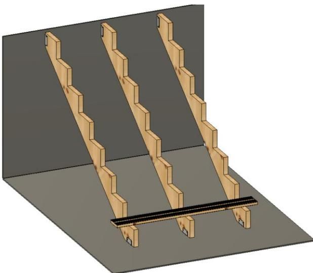
4- Screw the first plank on the first step with the RT-UT 5x60mm screws supplied with your kit. (Use 2 screws per plank and two planks per stringer).
