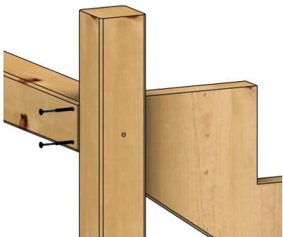
2. Place the support upright and align the stringer with the top of the support, the holes should be in the center of the stringer.
